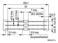
Minimum lead spacing 10 mm Approx. weight 0.25 g B78148T (central radial leads, taped)
